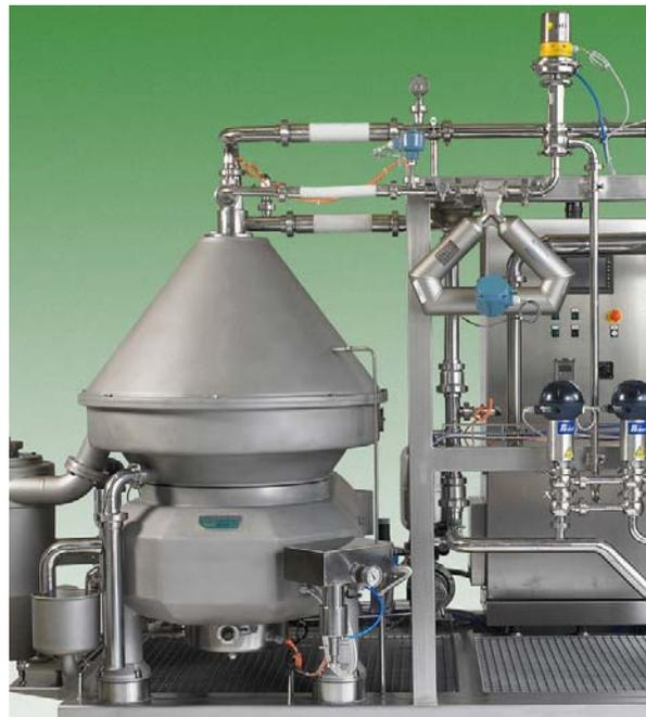
*Installation of an ELITE CMF100 meter on a standardization system used in milk separation and standardization*
