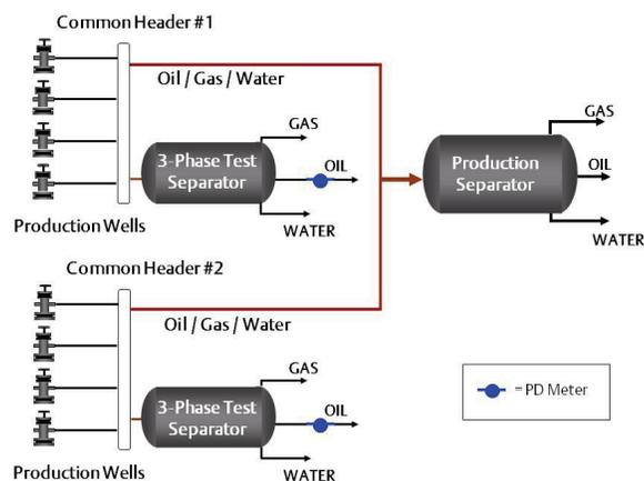
Positive displacement (PD) meter setup in large upstream production field
