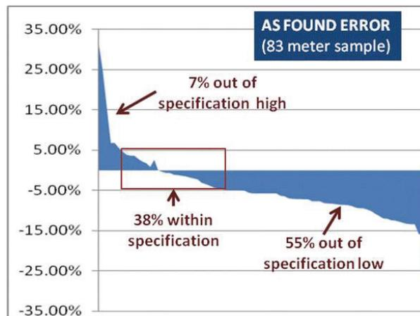
Test results for as found accuracy of PD meter sample
