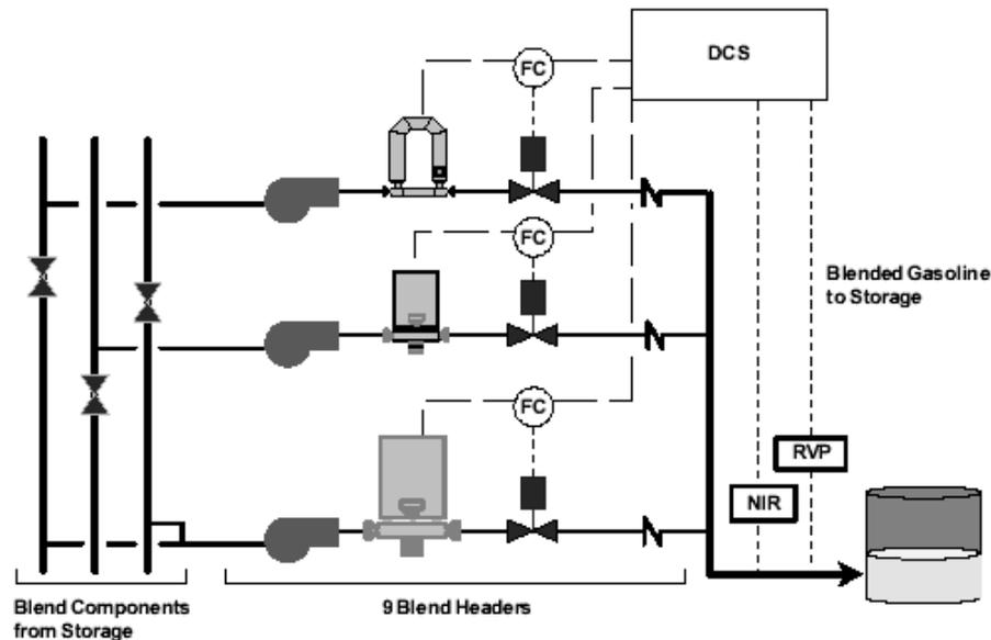
**Figure 1. Simplified gasoline blending schematic**
