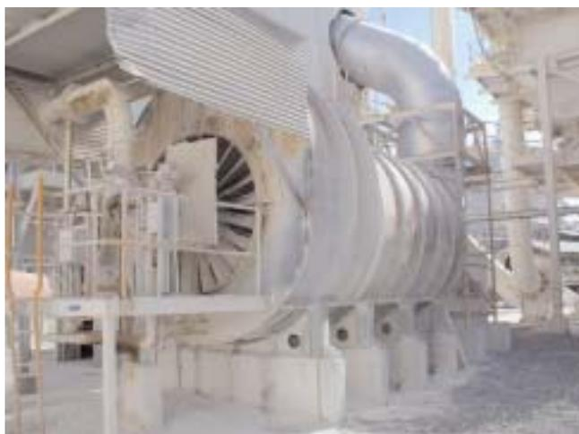
*Burners used in drying operations require between 6,000 to 90,000 cu ft per hour natural gas.*
