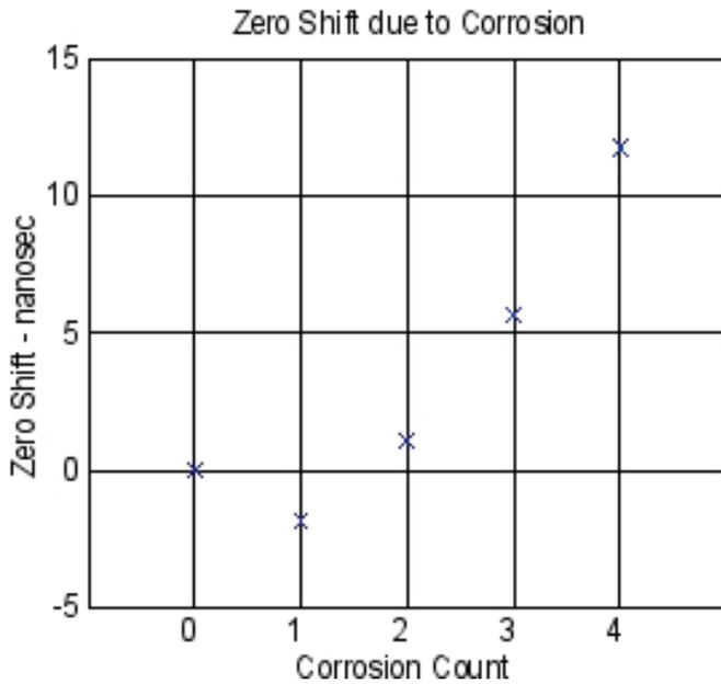
Figure 5. Zero Shift Due to Corrosion
