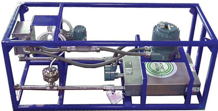
*Frac gel viscosity skid using Micro Motion Coriolis flow technology*
