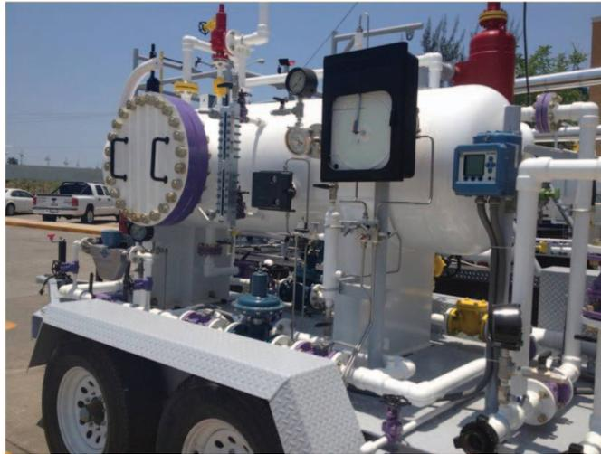
Mobile and compact oil separation system utilizing Micro Motion Coriolis technology
