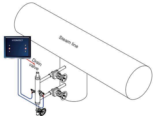
Figure 2. Automatically operated drain valve for bled steam lines
