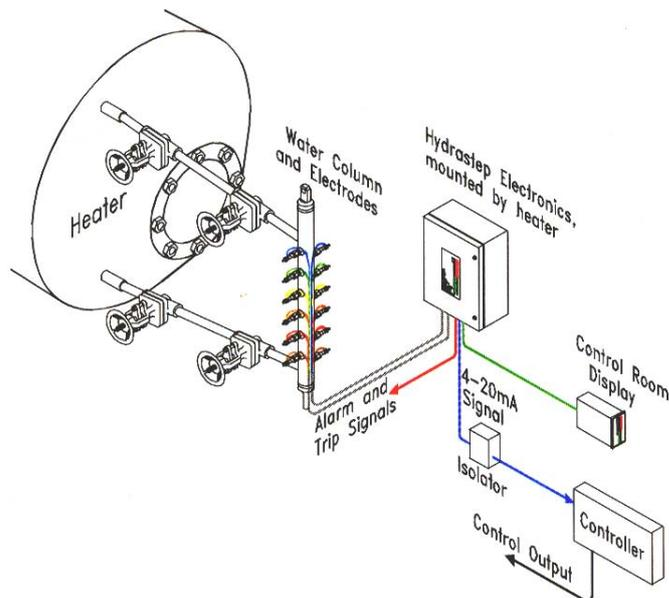
Heater control schemes can be greatly simplified by using Hydrastep for level control, and as heater level alarms and trips. Hydrastep's fully redundant system provides level alarms and analog outputs to create a completely reliable and repeatable level measurement system.
