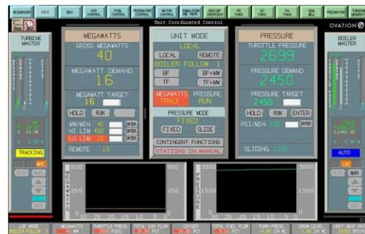
The Ovation system links the boiler and turbine controls through a coordinated front-end control strategy. This strategy can be implemented on either drum or supercritical boiler. Operators can use the coordinated control to generate and regulate the setpoint for unit load (MW) through local operator entry, remote increase/decrease contact inputs, or internally generated contingencies such as runbacks and rundowns.
