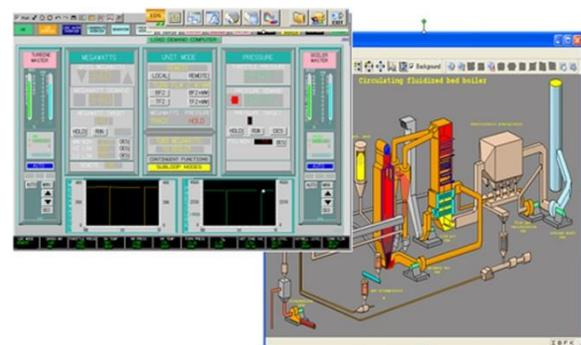
Figure 5: The EDS diagram display system supports up to 4 graphic windows.
