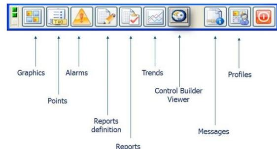
Figure 4: The EDS terminal toolbar for operations and I&C engineering
