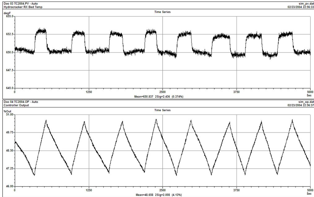
Figure 6: Limit cycle in Rx Bed Quench Temperature due to 3% valve stiction
