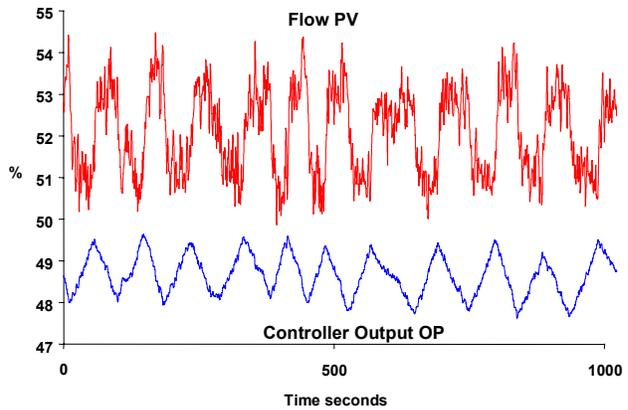
Figure 2: Limit cycle in a flow loop due to a sticky valve
