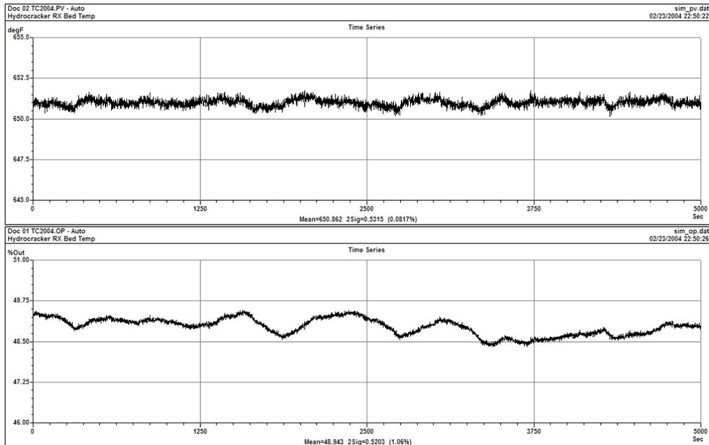
Figure 7: Reactor Bed Quench Temperature Control after improving valve performance
