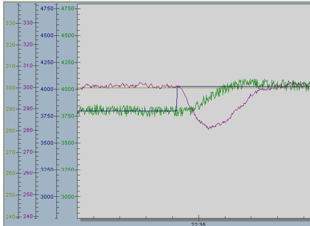
Figure 4: Desalter Flow and Pressure Interactions
