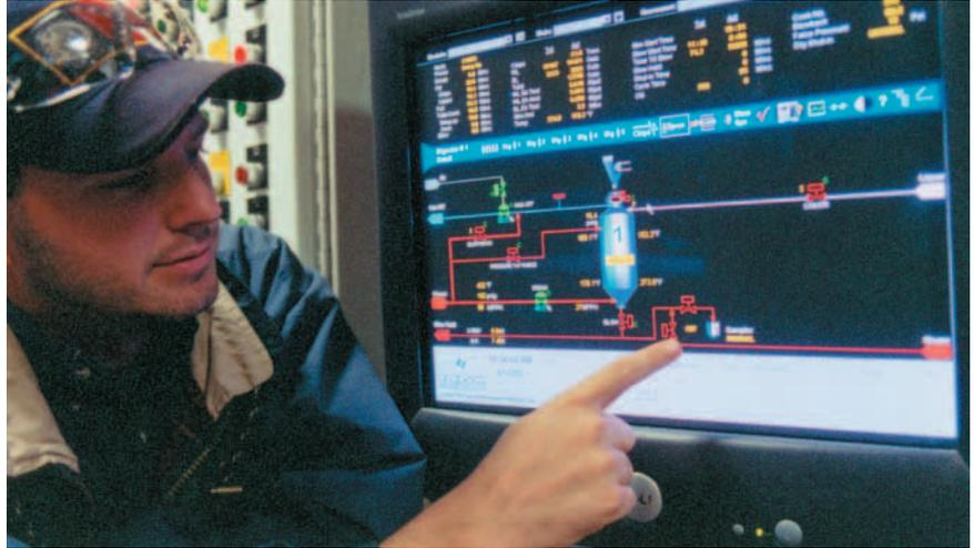
Because each Interstate digester has its own operating characteristics, the algorithms were customized to take these differences into account. As a result, finished pulp is highly consistent from digester to digester and batch to batch—less than 3% coefficient of variation. The control system's modified H-factor can also be simply raised or lowered across the entire digester house to accommodate variations among seasons, types of wood, and wood moisture content.
