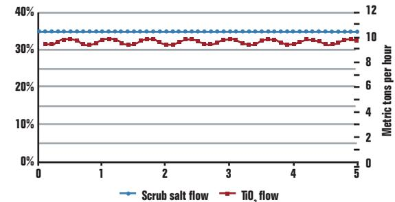
WITH CONTINUOUS INSTEAD OF ON-OFF SALT CONTROL, AVERAGE OUTPUT RISES FROM 6.7 TO 9 TPH. SALT CONSUMPTION HAS BEEN REDUCED 34% FROM AN AVERAGE OF 53% TO AN AVERAGE OF 35% OF MAXIMUM PUMP CAPACITY.
