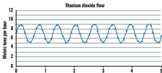
A TYPICAL OPERATOR TREND CHART OF THE REACTOR TiO<sub>2</sub> OUTPUT SHOWED CYCLIC VARIABILITY WITH FLOWS AVERAGING AROUND 6.7 TPH. THE DESIGN RATE WAS 7.0 TPH.
