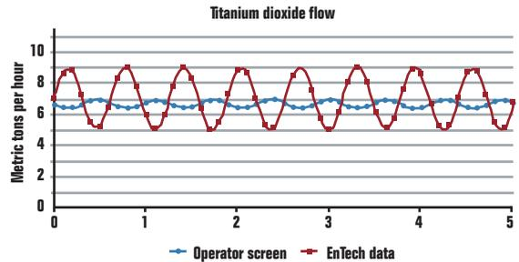
A LOOP AUDIT OF DATA FROM THE FINAL CONTROL ELEMENTS OVERLAID ON THE OPERATOR CHART (FIGURE 1) SHOWED THE SAME AVERAGE FLOWS AND PERIOD WITH THE CYCLES OUT OF PHASE BY 180 DEGREES, AND THE POTENTIAL FOR A PRODUCTION RATE OF MORE THAN 9 TPH.
