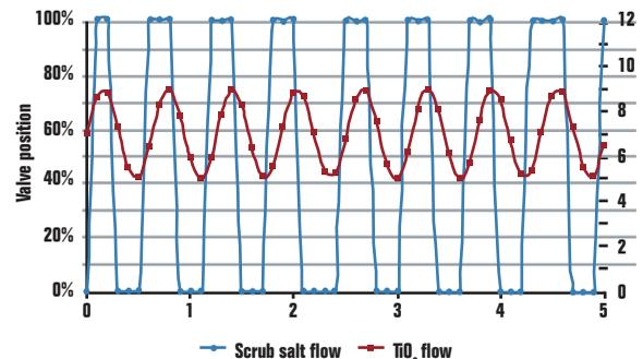
A FULL AUDIT SHOWED THE SCRUB SALT VALVE HAD THE SAME PERIOD AS REACTOR TiO<sub>2</sub> OUTPUT. WHEN THE VALVE WAS SWITCHED TO AN ARBITRARY CYCLE OF 25 SECONDS OPEN AND 23 SECONDS CLOSED, THE REACTOR OUTPUT TRACKED EXACTLY.
