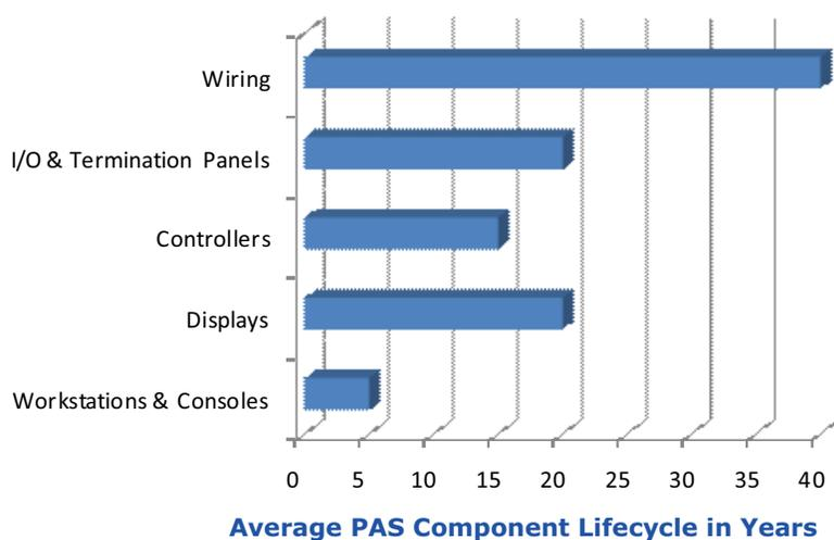
End users also have to look at the lifecycle of their system based on different tiers of longevity. Wiring, for example, typically has a lifecycle of 30 years or even longer. I/O and termination panels can last up to 20 years, while controllers typically have a shorter lifecycle of around 15 years, while workstations and consoles typically last around five years.
