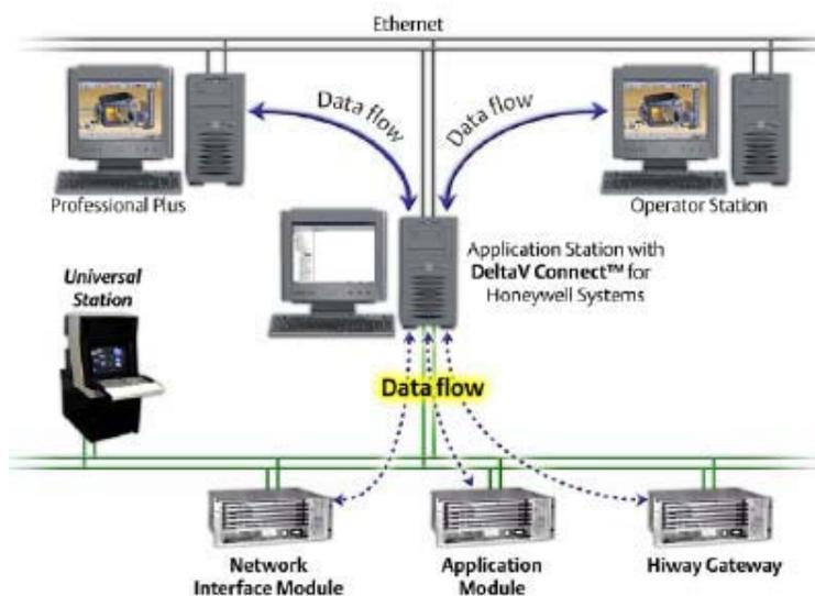
**The DeltaV Connect Solution for Honeywell Systems Sends and Receives DeltaV and Honeywell LCN Data**
