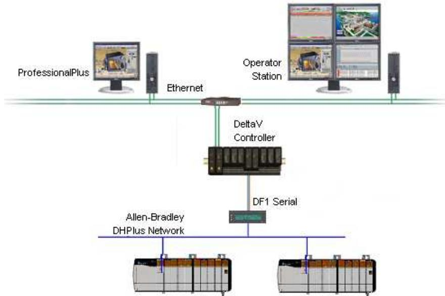
Figure 2— DeltaV™ serial connectivity to a PLC Network
