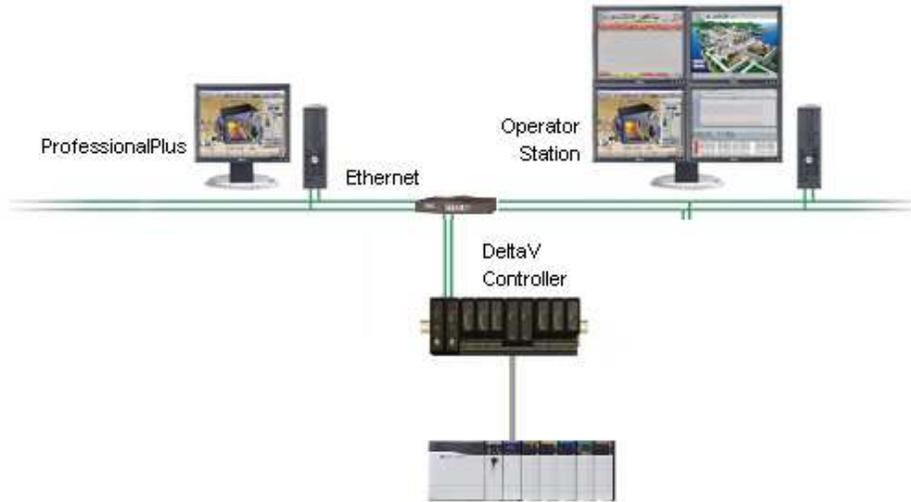
Figure 1— DeltaV™ serial connectivity to a PLC
