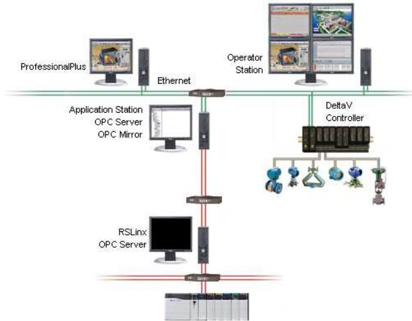
Figure 5— DeltaV™ OPC connectivity to a PLC
