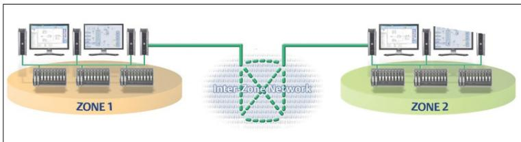
**Figure 2** Because the communication across zones was process critical, Preem chose to implement redundant inter-zone servers
