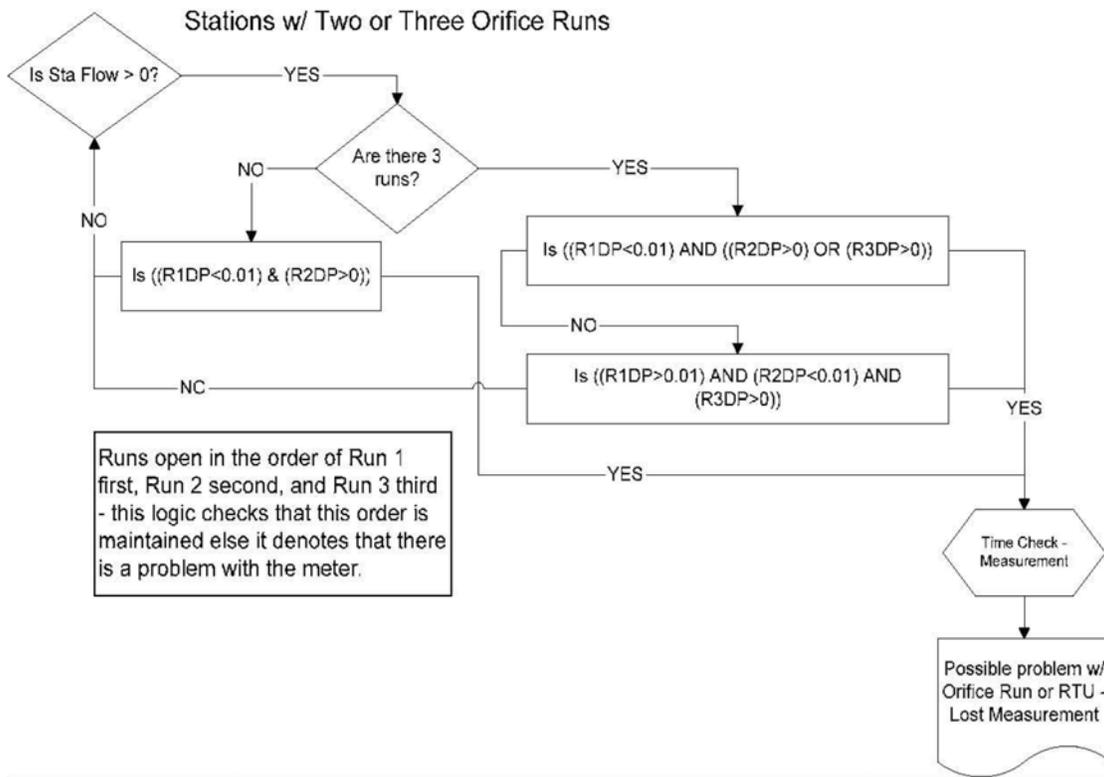
Figure 8. Meter Station Alarm
