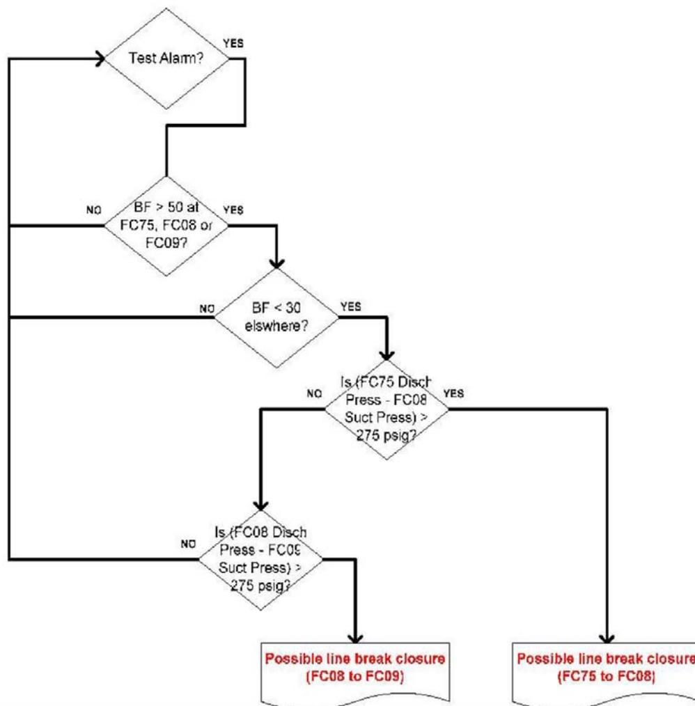
Figure 4. Line Break Operator Alarm
