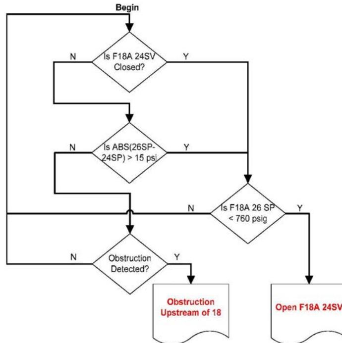
Figure 9. Station 18 Suction Valve Alarm
