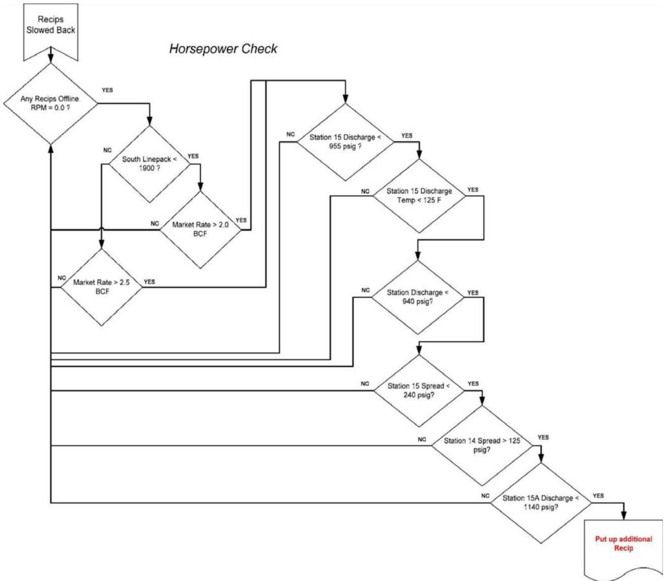
Figure 3. Additional Horsepower Required Alarm
