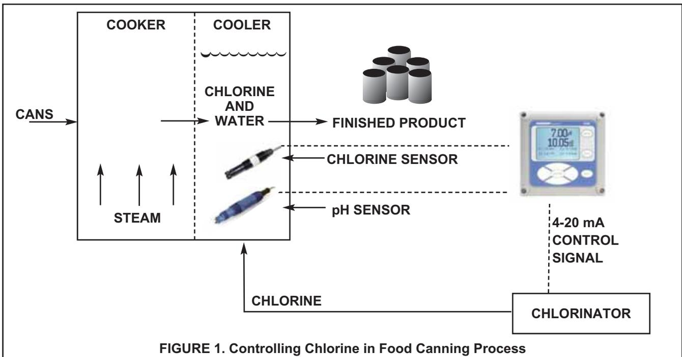
FIGURE 1. Controlling Chlorine in Food Canning Process
