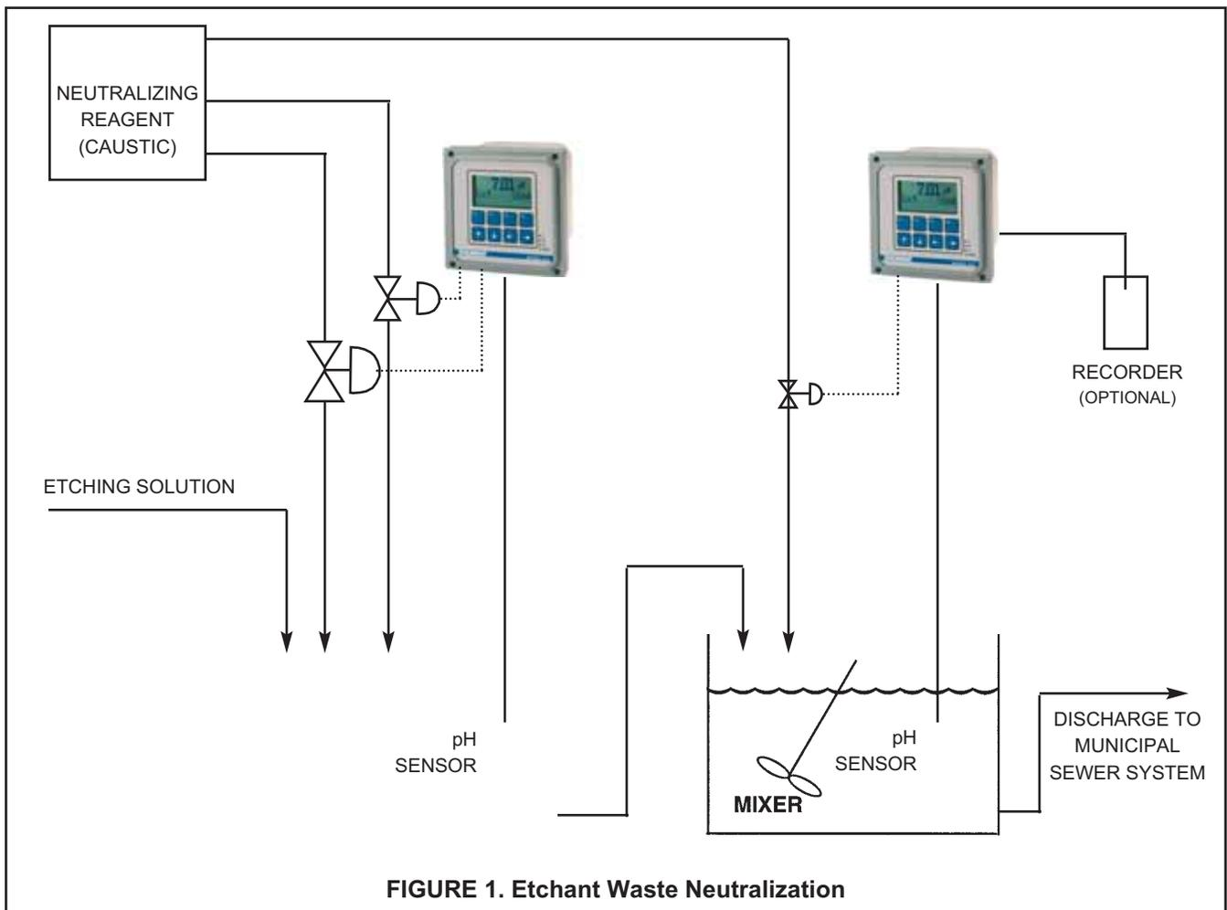
FIGURE 1. Etchant Waste Neutralization
