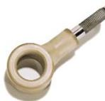
The Rosemount Analytical **Model 226** Toroidal Conductivity sensor is ideal for use in the slaker because its large 1.87 in. bore is not easily plugged by the heavy lime solids present. The sensor is injection molded of polyetheretherketone (PEEK) and comes complete with an integral temperature compensator.
