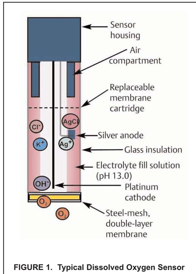
FIGURE 1. Typical Dissolved Oxygen Sensor
