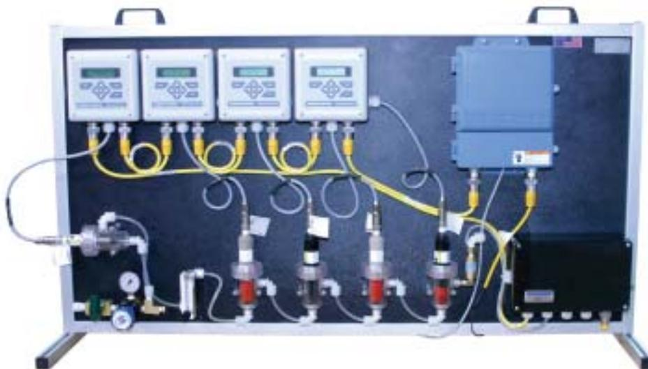
The Foundation Fieldbus based Water Quality System incorporates the Model 3420 FIM (Fieldbus Interface Module). The 3420 makes it possible to configure and diagnose Fieldbus transmitters via Ethernet using a web browser, and to data log the measurements via OPC over Ethernet and via Modbus.
