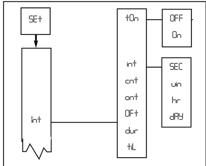
**Figure 4-2.** Interval Timer Configuration
