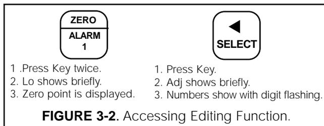
Configuration is all accomplished through a series of menus located within the set mode menu. To access these set mode menus the ACCESS keypad is pressed **TWICE** in **RAPID** succession.
