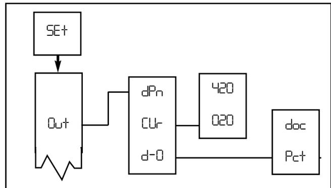
**Figure 4-4.** Current Output Configuration
