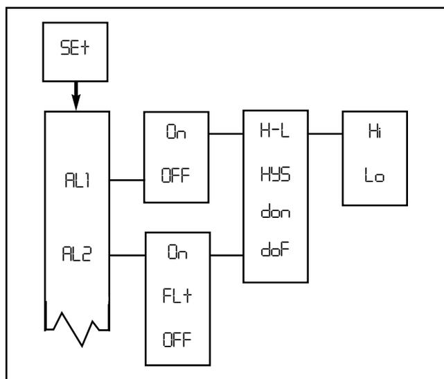
**Figure 4-1.** Alarm 1 and Alarm 2 Configuration
