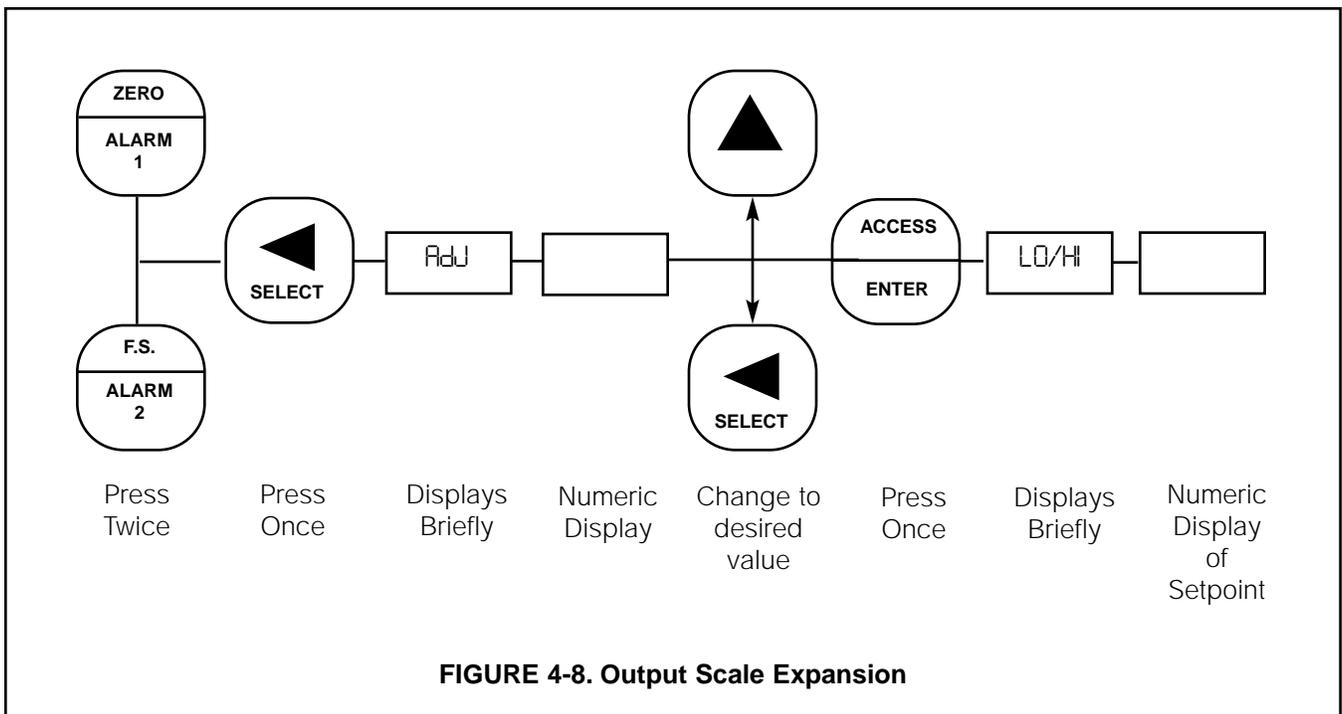
**FIGURE 4-8. Output Scale Expansion**
