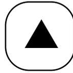
**B. SCROLL Key (▲).** This key is used to scroll through menu when selected, or scroll through digits on the active (flashing) Numeric Display, or move the decimal point and  $\mu\text{S}/\text{mS}$  display. Holding key down auto scrolls display.
