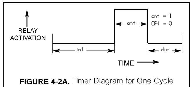
**FIGURE 4-2A.** Timer Diagram for One Cycle
