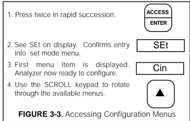
Once inside the Set mode menu, use the scroll keypad to scroll through the menu list. When the menu desired is displayed, release the scroll keypad.
