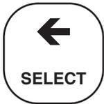
**A. SELECT/Shift (←) Key.** This key is used to select the displayed menu, or for shifting to the next digit in the Numeric Display.
