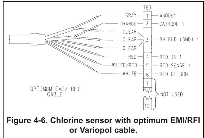
Figure 4-6. Chlorine sensor with optimum EMI/RFI or Variopol cable.
