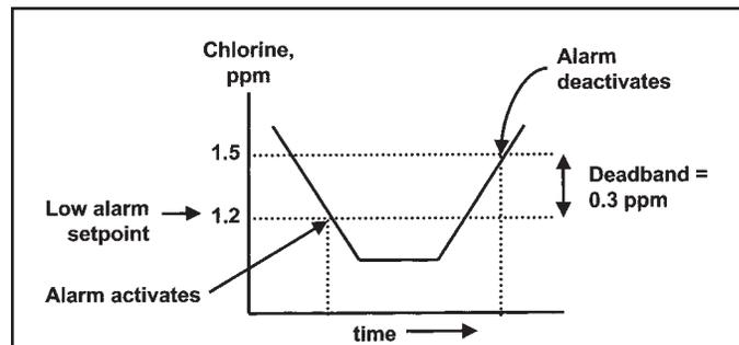
**FIGURE 7-2. Low Alarm Logic**
