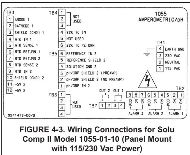
**FIGURE 4-3. Wiring Connections for Solu Comp II Model 1055-01-10 (Panel Mount with 115/230 Vac Power)**
