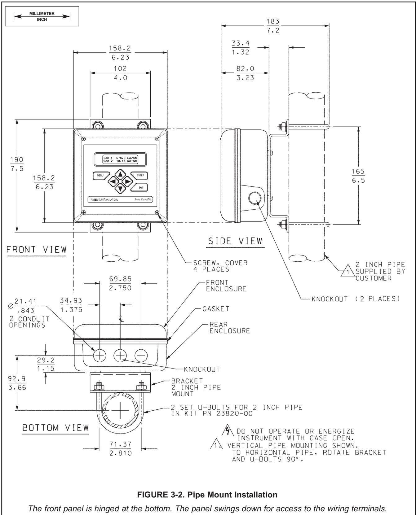
**FIGURE 3-2. Pipe Mount Installation**
