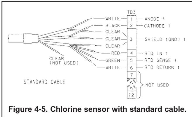
Figure 4-5. Chlorine sensor with standard cable.
