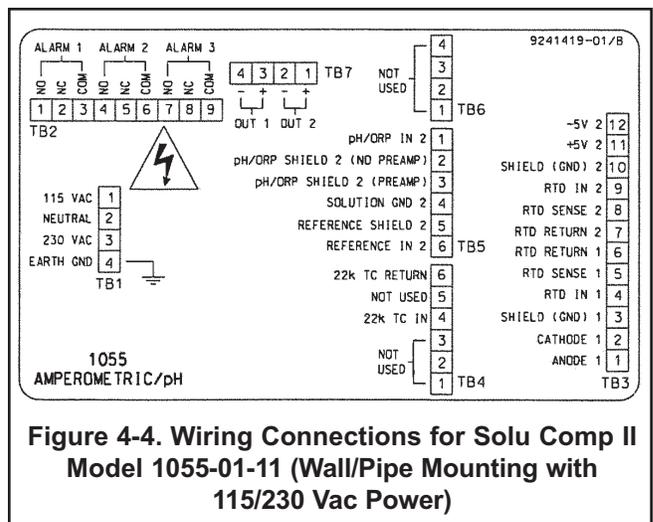
**Figure 4-4. Wiring Connections for Solu Comp II Model 1055-01-11 (Wall/Pipe Mounting with 115/230 Vac Power)**
