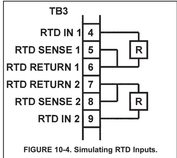
FIGURE 10-4. Simulating RTD Inputs.
