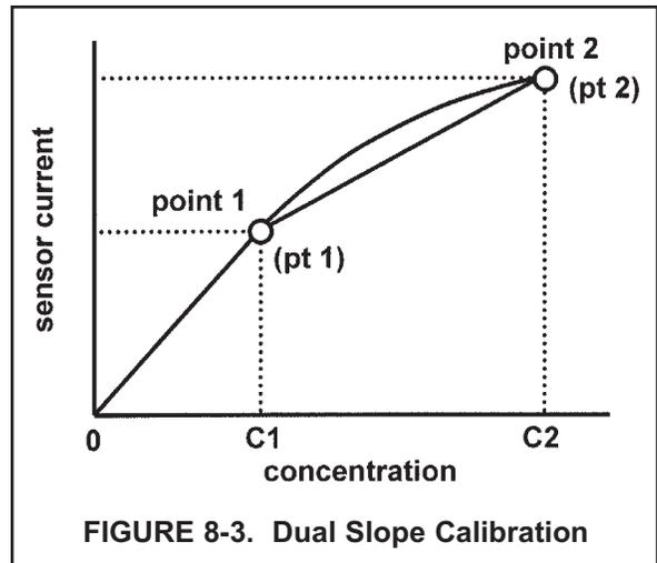
**FIGURE 8-3. Dual Slope Calibration**
