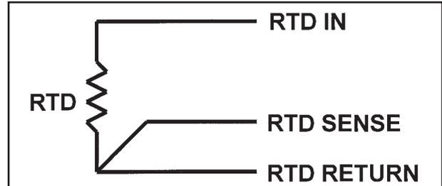
FIGURE 10-3. Three-Wire RTD Configuration.
