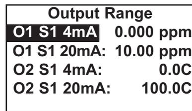
5. The screen at left appears. The screen shows the present values assigned to output 1 (**O1**) and output 2 (**O2**). The screen also shows which sensors the outputs are assigned to. **S1** is sensor 1 and **S2** is sensor 2. **S2** appears only if you have a dual input 1056 analyzer. The assignments shown are the defaults for a single channel chlorine analyzer. Outputs are freely assignable under the configure menu.
