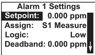
5. The screen summarizes the present configuration and setpoints. There are nine items: **Setpoint, Assign (S1 is sensor 1 and S2 is sensor 2), Logic, Deadband, Interval time, On time, Recover time, and Hold while active**. The last four items describe the operation of the timer. Only four items are shown at a time. To view the remaining items, scroll to the bottom of the screen and continue scrolling.
