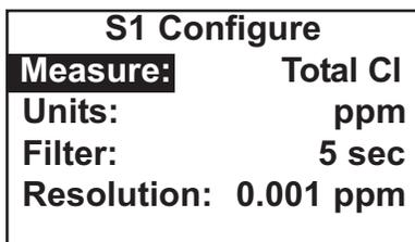
4. The screen summarizes the present configuration for the chlorine sensor. There are four items: **Measure**, **Units**, **Filter**, and **Resolution**
