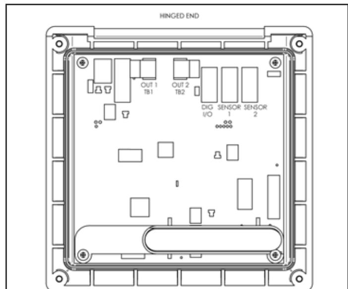
**FIGURE 4-2. Analog output connections.** The analog outputs are on the main board near the hinged end of the enclosure door.
