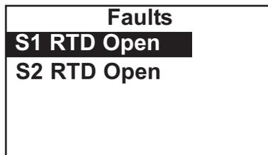
2. If you choose **Fault** or **Warning**, a screen like the one shown at left appears. **S1** means sensor 1. **S2** means sensor 2. For additional troubleshooting information, select the desired message and press ENTER. For more information, see Section 11.3.
