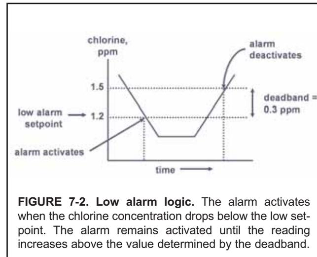
**FIGURE 7-2. Low alarm logic.** The alarm activates when the chlorine concentration drops below the low setpoint. The alarm remains activated until the reading increases above the value determined by the deadband.
