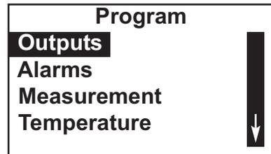
2. To assign values to the analog outputs, the **Program** sub-menu must be open. Use the down navigation key to move the cursor to **Program**. Press ENTER.
