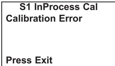
If the sensitivity is too far outside the range of expected values, the calibration error screen shown at left will appear. The analyzer will not update the calibration. For troubleshooting assistance, see Section 11.5.
