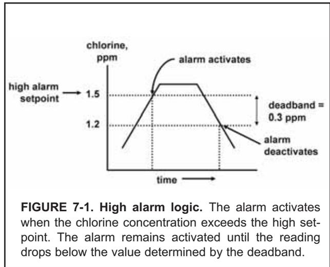
**FIGURE 7-1. High alarm logic.** The alarm activates when the chlorine concentration exceeds the high setpoint. The alarm remains activated until the reading drops below the value determined by the deadband.
