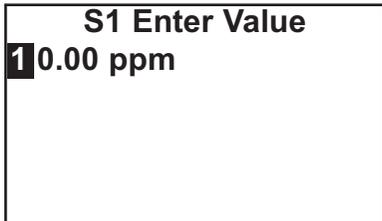
Determine the total chlorine concentration in the sample and enter the value in the screen shown at left. See Section 9.3.1 for sampling and testing precautions.
