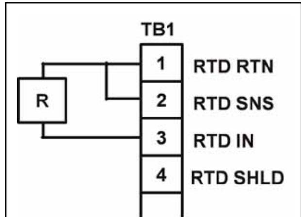
FIGURE 11-4. Simulating RTD Inputs.
