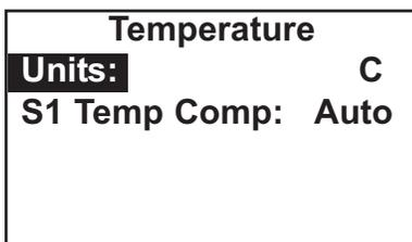
3. The screen summarizes the present sensor configuration. There will be between two and five items. **Units** and **S1 Temp Comp**, always appear. If manual temperature compensation was selected, the manual temperature value will also appear. If you have a dual input analyzer, temperature compensation items will appear for the other sensor. Only four items are shown at a time. To view the remaining items, scroll to the bottom of the screen and continue scrolling.
