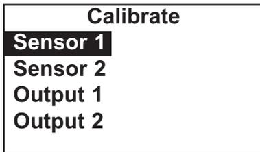
4. Choose the sensor you wish to calibrate. **Sensor 2** appears only if you have a dual input 1056 analyzer.
