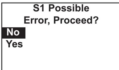
If the zero current is moderately larger than expected, an error message appears. To force the analyzer to accept the zero current, choose **Yes**. To repeat the calibration, choose **No**. For troubleshooting assistance, see Section 11.5.
