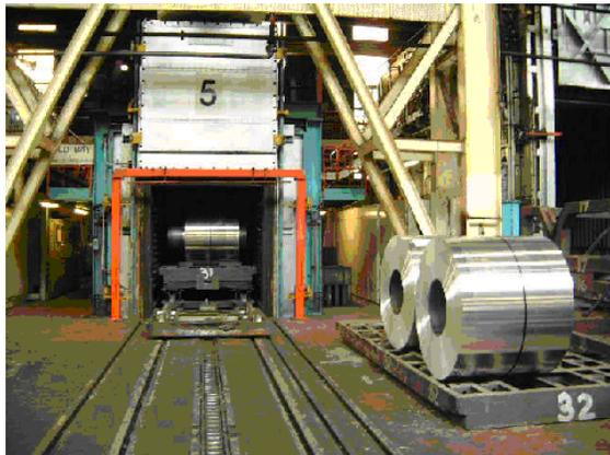
Cold rolled metal products must be annealed after rolling to eliminate work stresses induced by the rolling process. Usually some amount of “grain growth” is caused by the rolling process, depending on the amount of cross-sectional reduction accomplished. Various furnace types are utilized to execute the annealing process, which raises the metal temperature to a point where the crystalline structure is returned to normal.
