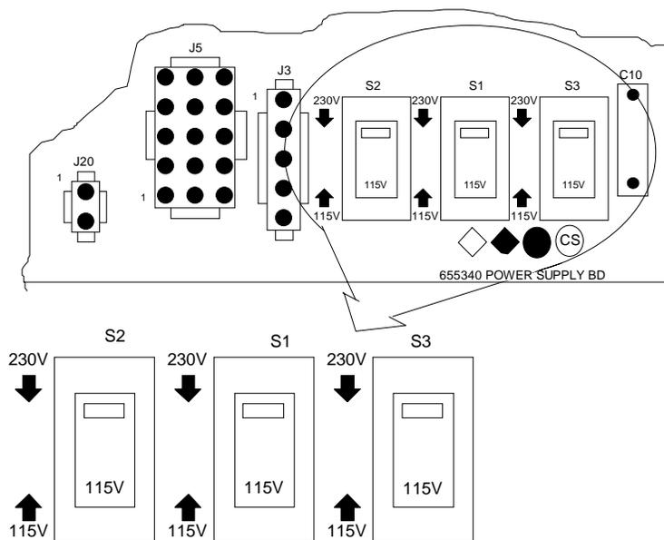
Set switch window for voltage required.
