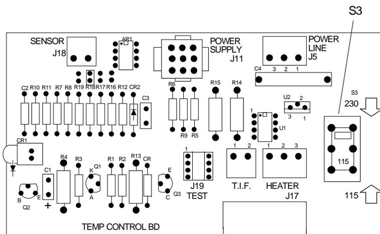
Set switch window for voltage required.
