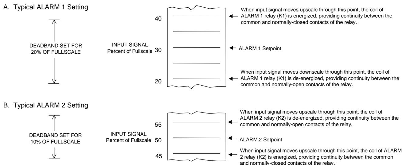
**FIGURE 2-5. TYPICAL ALARM SETTINGS**
