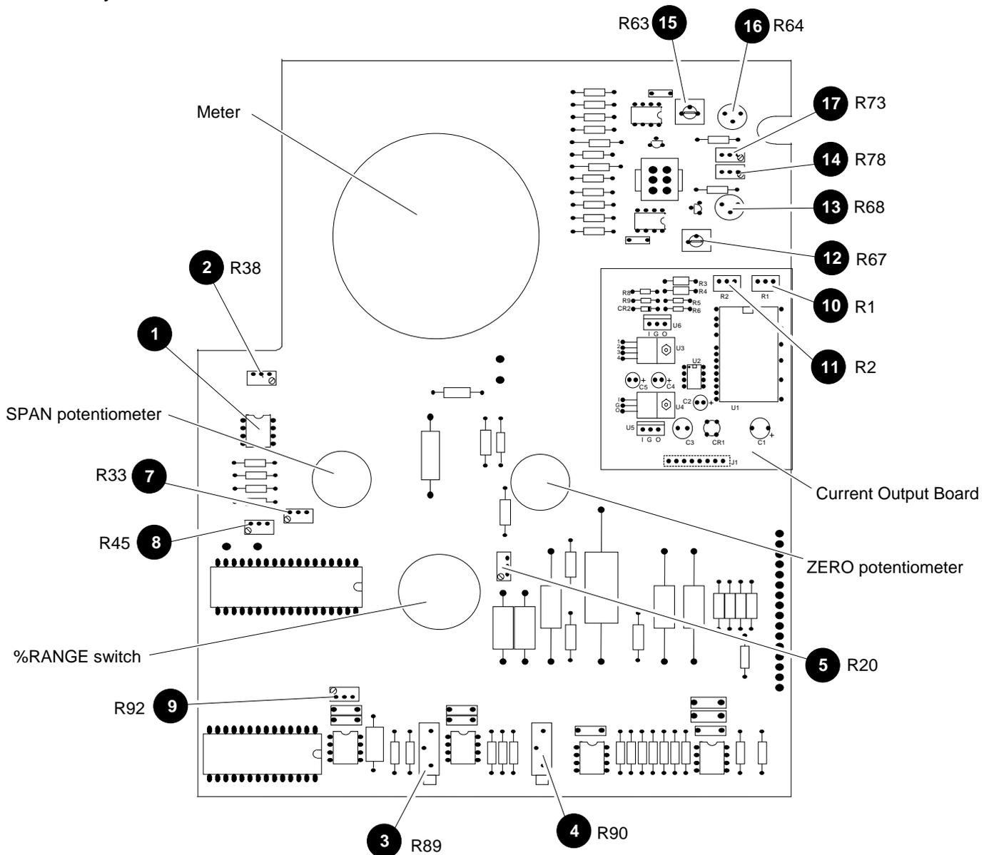
**FIGURE 3-1. CONTROL BOARD - ADJUSTMENT LOCATIONS**
