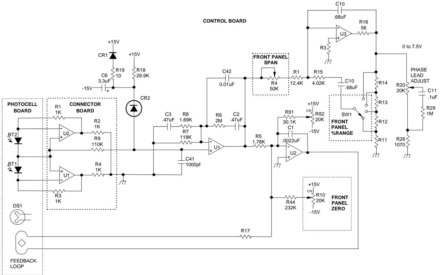
**FIGURE 6-6. DETECTOR WITH FIRST STAGE AMPLIFIER**
