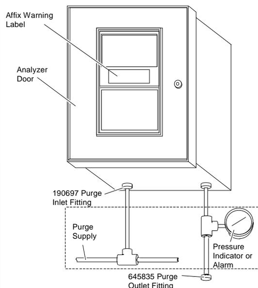
Components in dashed line are supplied by customer.
