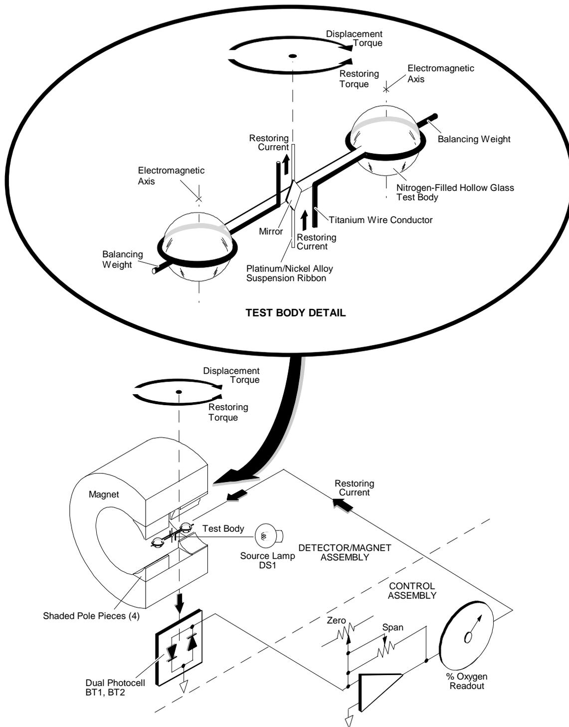
**FIGURE 5-1. FUNCTIONAL DIAGRAM OF MODEL 755 PARAMAGNETIC OXYGEN MEASUREMENT SYSTEM**
