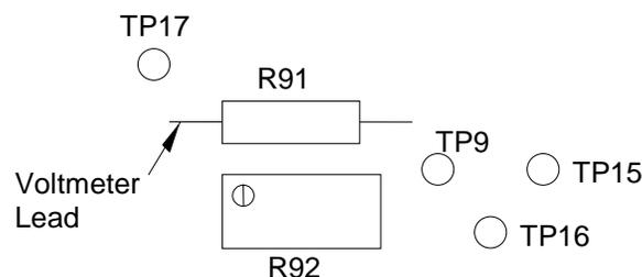
**FIGURE 7-7. PHOTOCCELL ADJUSTMENT VOLTMETER LEAD LOCATION**
