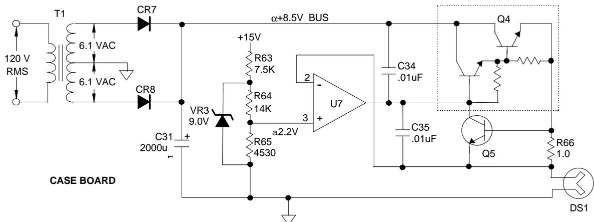
**FIGURE 6-5. DETECTOR LIGHT SOURCE CONTROL CIRCUIT**
