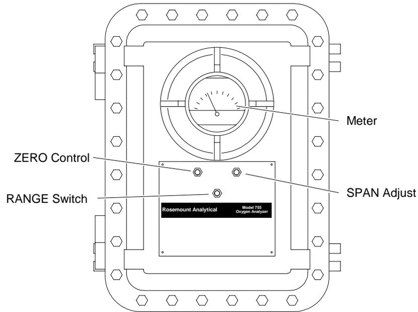
Controls have slotted shafts for screwdriver adjustment from outside the enclosure.
