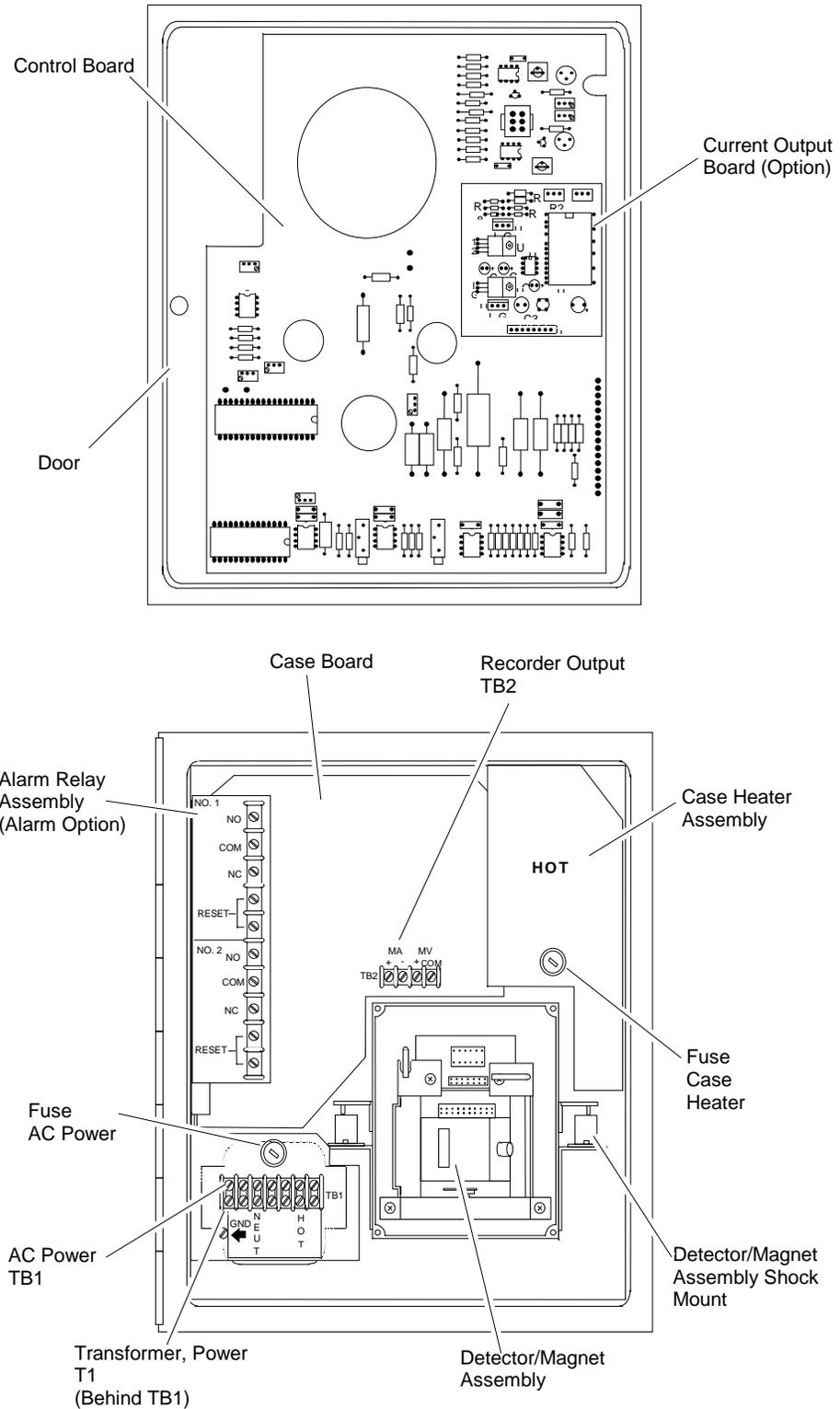
General Purpose enclosure shown. Components mounted in same locations in Explosion-Proof enclosure.
