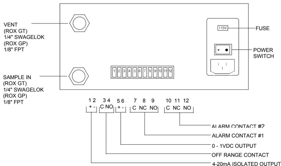
Figure 2-2. Back Panel Connections
