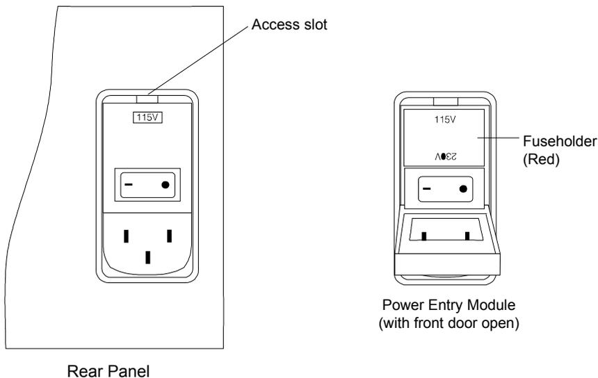
**Figure 4-2. ROX GT, GP 115/230V AC Fuse Location**
