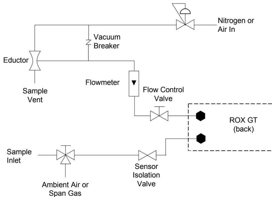
Figure 2-4. Recommended Sample Handling Diagram - Insufficient Pressure or Flow
