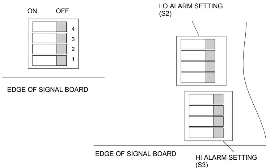
**Figure 4-4. Alarm Switch Location**
