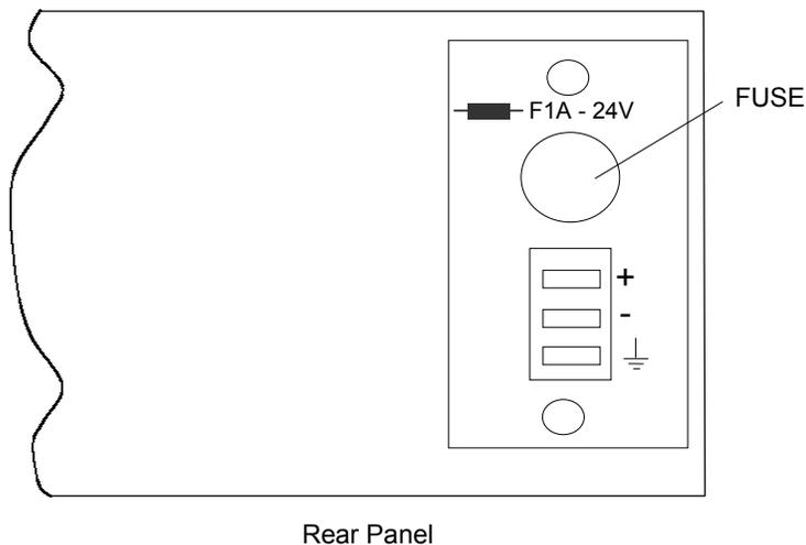
**Figure 4-3. ROX GT 24V DC Fuse Location**
