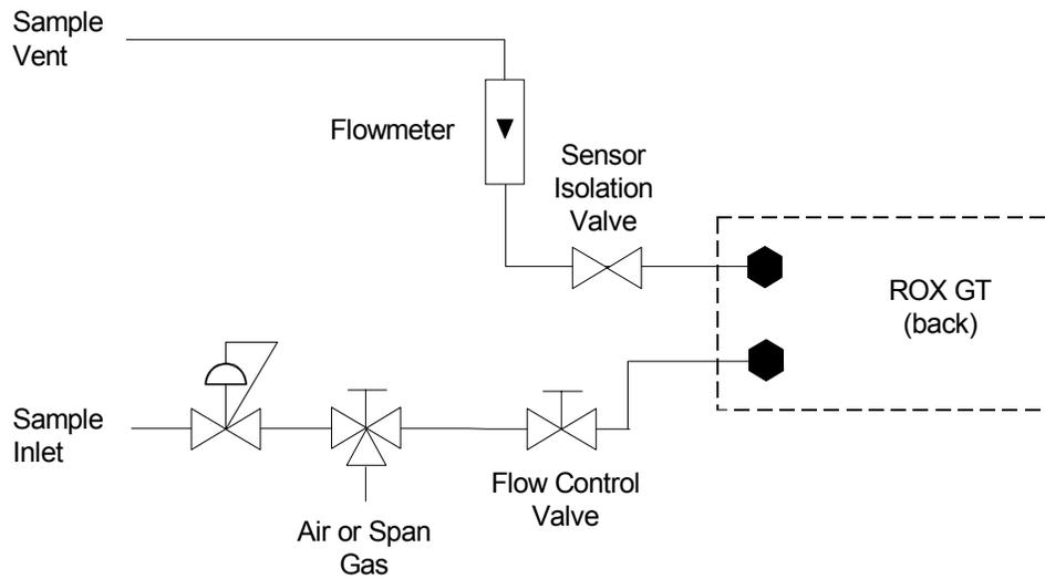
Figure 2-3. Recommended Sample Handling Diagram - Positive Pressure Sample
