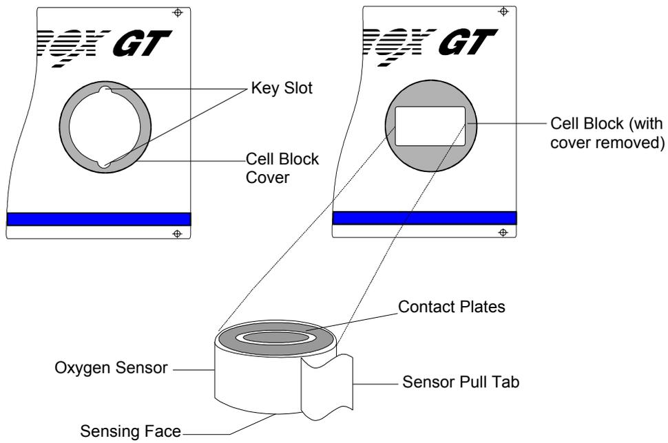
**Figure 4-1. Sensor Installation**
