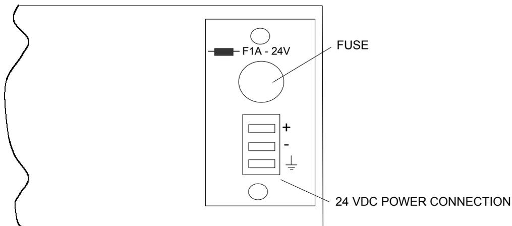
**Figure 2-5. Rear Panel Electrical Input Connection**
