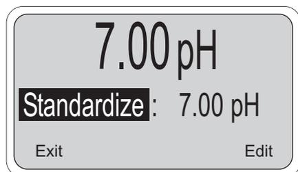
7. The pH reading in large numbers is the current process reading. Press Edit (F4). Use the arrow keys to change the reading in the second line to match the referee instrument. Press Save (F4).
