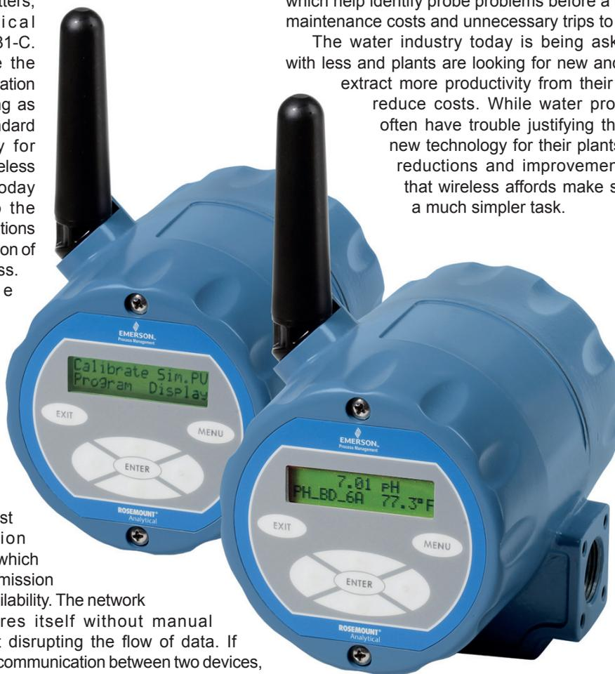
**Rosemount® Analytical's wireless field instrument solutions include both conductivity and pH/ORP measurement. Shown here are the wireless pH and ORP transmitter 6081-P and the 6081-C, a wireless conductivity transmitter.**
