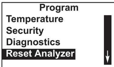
2. Scroll to the bottom of the screen and continue scrolling until **Reset Analyzer** is highlighted. Press ENTER.
