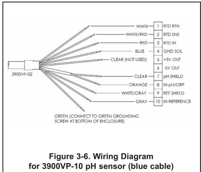
**Figure 3-6. Wiring Diagram for 3900VP-10 pH sensor (blue cable)**
