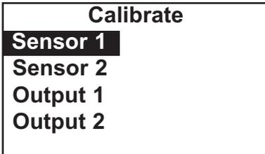
4. Choose the sensor you wish to calibrate. **Sensor 1** is the chlorine sensor. **Sensor 2** (if present) is the pH sensor.
