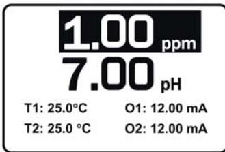
3. **Main Format** lets you configure the second line in the main display as well as the four smaller items at the bottom of the display. Move the cursor to the desired place in the screen and press ENTER. Scroll through the list of items and select the parameter you wish displayed. Once you are done making changes, press EXIT twice to return to the display menu. Press MENU then EXIT to return to the main display.
