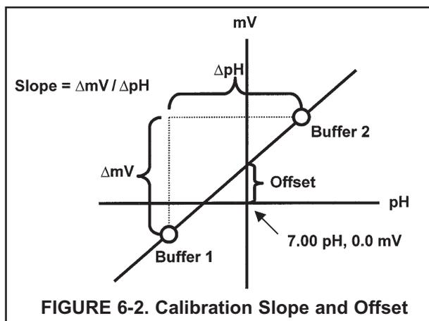
5. USER ENTERED SLOPE AND OFFSET. If the slope and offset are known from other measurements, they can be directly entered in the analyzer. Enter the slope as a positive number corrected to 25°C. To calculate the slope at 25°C from the slope at temperature t°C, use the equation:
