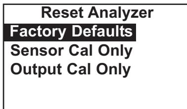
3. Choose whether to reset all user-entered values (**Factory Defaults**), sensor calibration (**Sensor Cal Only**), or output calibration (**Output Cal Only**). If you choose **Sensor Cal Only** or **Output Cal Only** a second screen appears in which you can select which sensor or output calibration to reset.
