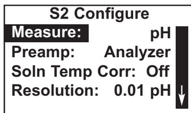
5. The screen summarizes the present configuration for sensor 2 (pH). There are six items: **Measure**, **Preamp**, **Sol'n Temp Corr**, **Resolution**, **Filter**, and **Reference Z** (reference impedance). Only four items are shown at a time. To view the remaining items, scroll to the bottom of the screen and continue scrolling.
