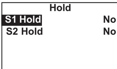
3. The screen shows the current hold status for each sensor. Select the sensor to be put in hold. Press ENTER.
