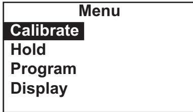
1. Press MENU. The main menu screen appears. There are four items in the main menu. **Calibrate** is in reverse video, meaning that the cursor is on Calibrate.
