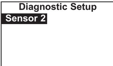
3. Diagnostics are available only for pH sensors. In the FCLi-02 the pH sensor is sensor 2. Press ENTER.
