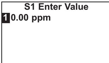
7. Follow the screen prompts: Once the reading is stable, press ENTER. Take the sample and press ENTER. At this point, the analyzer will store the present sensor current and temperature and use those values in the calibration.
