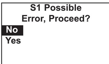
If the zero current is moderately larger than expected, an error message appears. To force the analyzer to accept the zero current, choose **Yes**. To repeat the calibration, choose **No**. For troubleshooting assistance, see Section 9.5.
