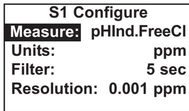
4. The screen summarizes the present configuration for sensor 1 (chlorine). There are four items: **Measure**, **Units**, **Filter**, and **Resolution**
