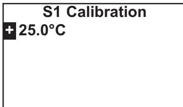
6. Change the display to match the temperature read from the calibrated thermometer. Press ENTER.
