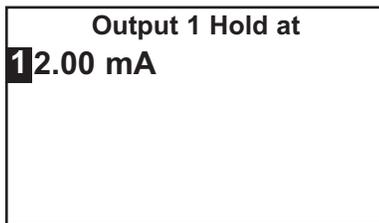
5. Enter the desired simulated output current. To end the simulated current, press MENU or EXIT.
