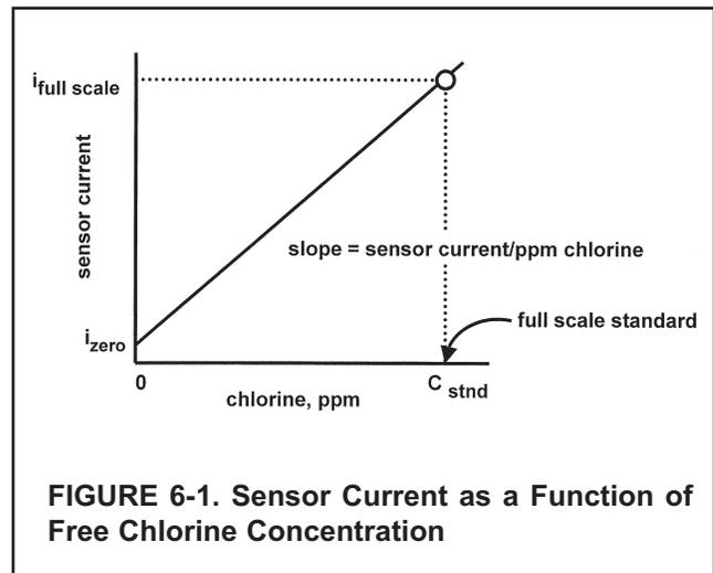
**FIGURE 6-1. Sensor Current as a Function of Free Chlorine Concentration**
