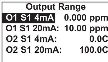
5. The screen at left appears. The screen shows the present values assigned to output 1 (**O1**) and output 2 (**O2**). The screen also shows which sensors the outputs are assigned to. **S1** is sensor 1 and **S2** is sensor 2. The assignments shown are the defaults for the FCLi-01. For the FCLi-02, Output 2 is assigned to sensor 2 (pH). Outputs are freely assignable under the configure menu.
