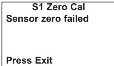
If the zero current is much larger than expected, the zero calibration failure screen appears. The analyzer will not update the zero current. For troubleshooting assistance, see Section 9.5.
