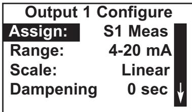
5. The screen shows the present configuration. There are six items: **Assign** (**S1** is sensor 1, **S2** is sensor 2), **Range**, **Scale**, **Dampening**, **Fault Mode**, and **Fault Value**. To display the fifth and sixth items, scroll to the bottom of the screen and continue scrolling.
