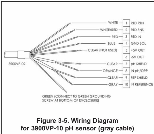
**Figure 3-5. Wiring Diagram for 3900VP-10 pH sensor (gray cable)**
