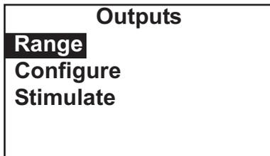
4. The screen at left appears. The cursor is on **Range**. **Output Range** is used to assign values to the low and high current outputs. Press ENTER.
