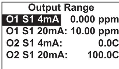
5. The screen shows the present settings for the outputs. **O1** is output 1, **O2** is output 2, **S1** is sensor 1, and **S2** is sensor 2.
