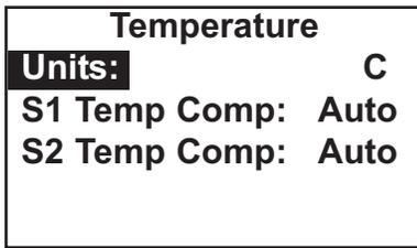
3. The screen summarizes the present sensor configuration. There will be between three and five items. **Units**, **S1 Temp Comp**, and **S2 Temp Comp** always appear. If manual temperature compensation was selected, the manual temperature values entered for each sensor (**S1 and S2 Manual**) will also appear. Only four items are shown at a time. To view the remaining items, scroll to the bottom of the screen and continue scrolling.
