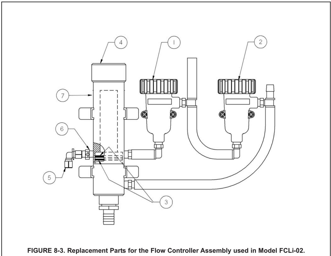
**FIGURE 8-3. Replacement Parts for the Flow Controller Assembly used in Model FCLi-02.**
