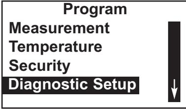
2. Scroll to the bottom of the screen and continuing scrolling until **Diagnostic Setup** is highlighted. Press ENTER.
