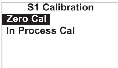
6. Choose **Zero Cal**. The analyzer will automatically start the zero calibration
