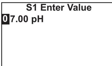
7. Once reading is stable, measure the pH of the liquid using a referee instrument. Because the pH of many natural and treated waters depends on temperature, measure the pH of the sample immediately after taking it. For poorly buffered samples determine the pH of a continuously flowing sample from a point as close as possible to the sensor.
