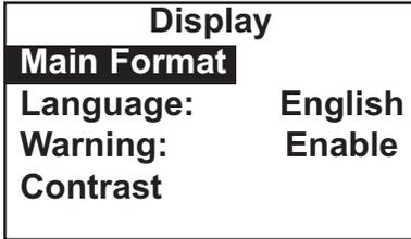
To make a change, move the cursor to the desired line and press ENTER. A screen appears in which the present setting can be edited. Press ENTER to store the setting.
