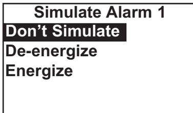
5. Choose **Don't simulate**, **De-energize**, or **Energize**. Press MENU or EXIT to end simulation.
