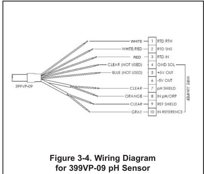
**Figure 3-4. Wiring Diagram for 399VP-09 pH Sensor**
