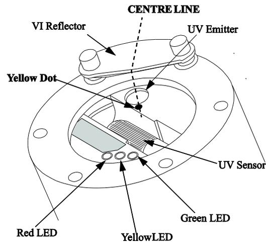
**Note:** An optional heater is available to eliminate condensation on the glass window/lens.
