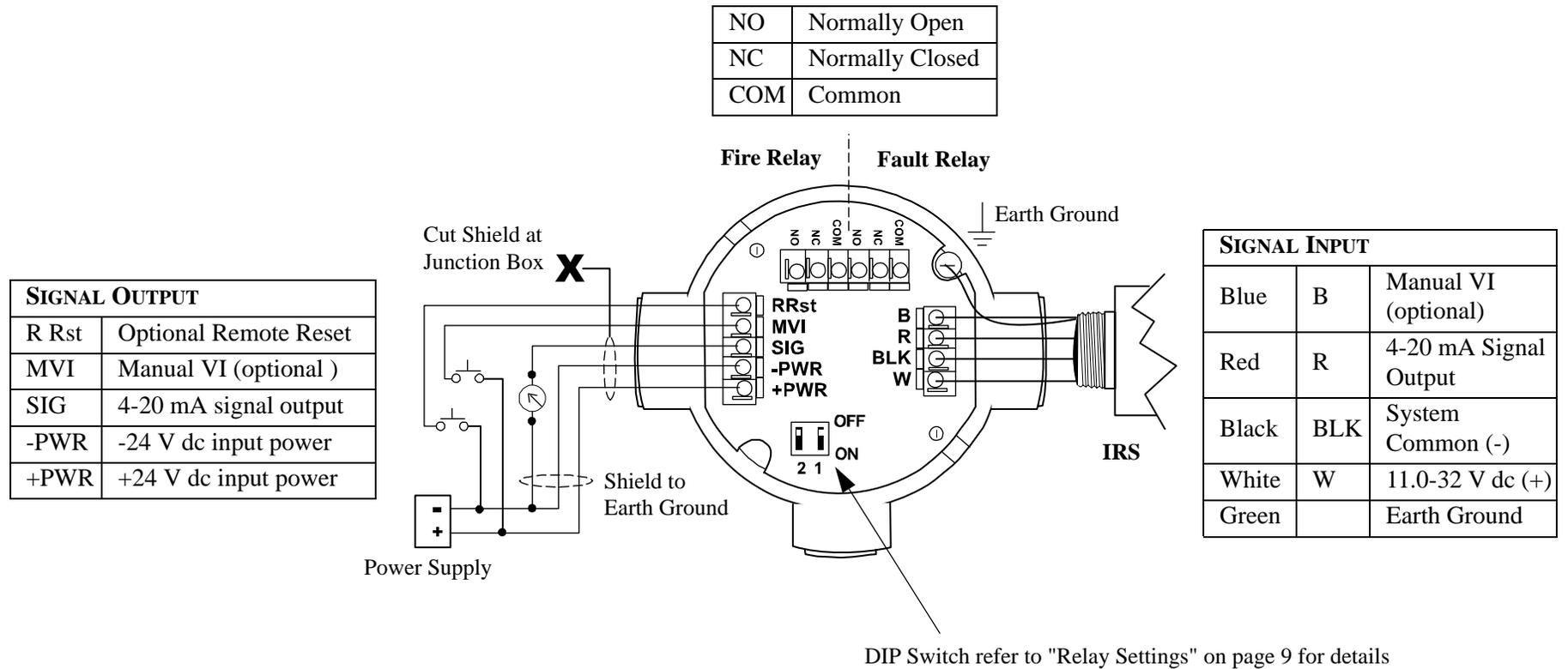
**Note:** If the 4-20 mA signal is not used, connect a jumper between the terminals for 4-20 mA signal output (SIG) and -24 V dc input power (-PWR) on the Signal Output terminal block.
