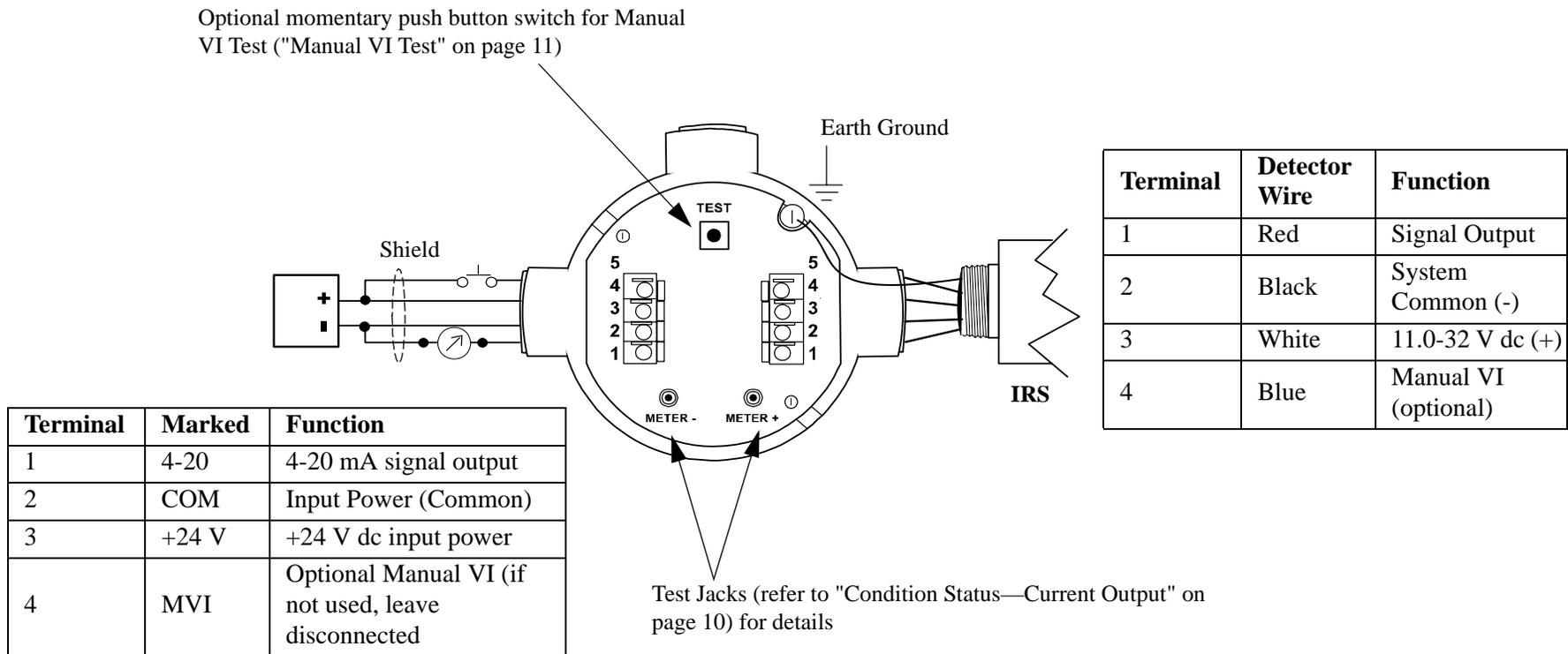
**Figure 5: Junction Box Connection — ANALOG/RELAY**
