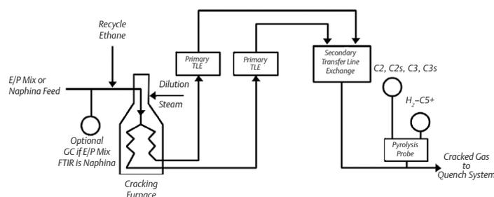
After the transfer line exchanges, the sample is cooled even more with oil-quenching and water-quenching systems. The cooled furnace effluent is compressed to an optimum pressure for separating into the various chemical components in the fractionation section where product recovery occurs. The stream is also run through a caustic wash system to remove H<sub>2</sub>S and CO<sub>2</sub> between compression stages.
