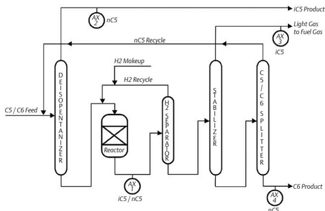
At the  $C_5/C_6$  splitter, the  $C_5$  are sent out the top of the tower and are recycled back to the beginning of the process unit. The  $nC_5$  in the  $C_5$  will be reprocessed while the  $iC_5$  will leave the top of the deisopentimizer as finished  $iC_5$  product. The  $C_6$  and heavier components leave the bottom of the splitter and either go to gasoline blending or to the reformer unit to be made into aromatics.
