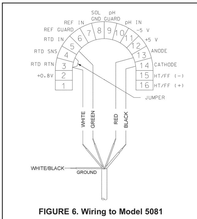
FIGURE 6. Wiring to Model 5081
