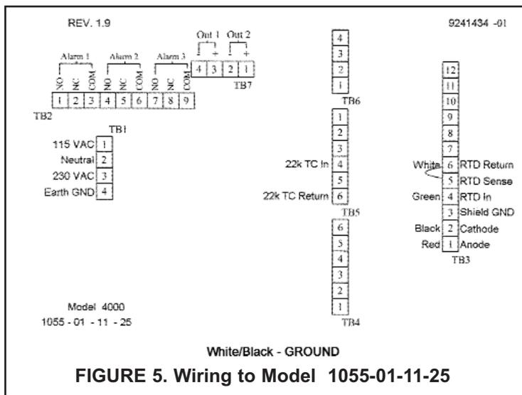
FIGURE 5. Wiring to Model 1055-01-11-25
