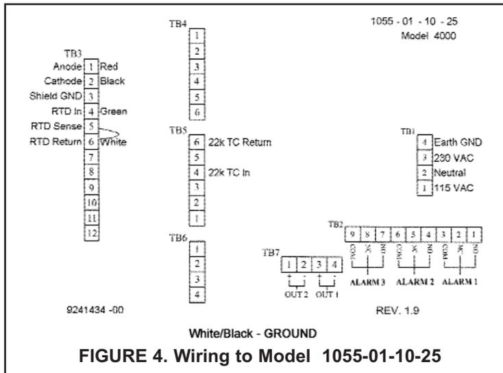
FIGURE 4. Wiring to Model 1055-01-10-25
