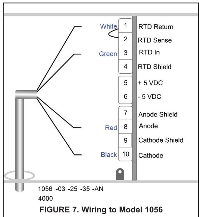
FIGURE 7. Wiring to Model 1056
