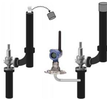
*A "sock off" situation (left) automatically assumed a 12 hour VOC emission at the maximum release rate. New wireless instruments from Emerson (right) provide trend data that can help operators prevent VOC emissions.*
