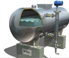
**Guided Wave Radar is immune to density changes and provides a low maintenance alternative to displacers.**
