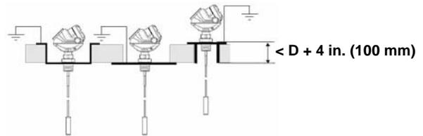
**Installation in concrete silo with metal shielding**
