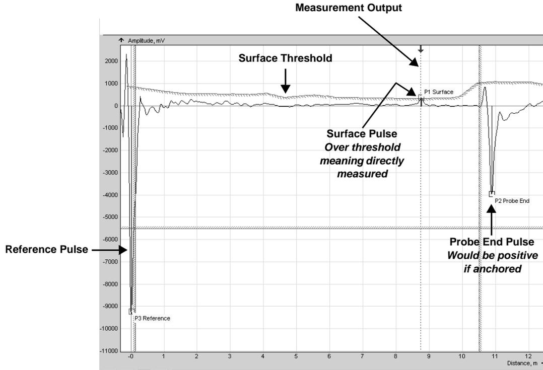
(a) Echo Curve Showing Surface Directly Measured
