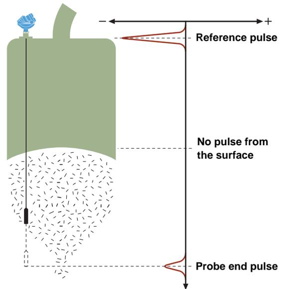
The PEP function is recommended for solids with a dielectric constant less than or equal to 2. The maximum measuring range with PEP is 164 ft. (50 m) (maximum probe length) divided by the square root (sqrt) of the material dielectric constant (DC) + the air gap to the material surface.
