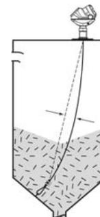
**Fixing probe with slack**
