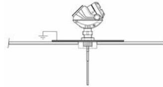
**Installation with metal sheet in non-metallic vessels**
