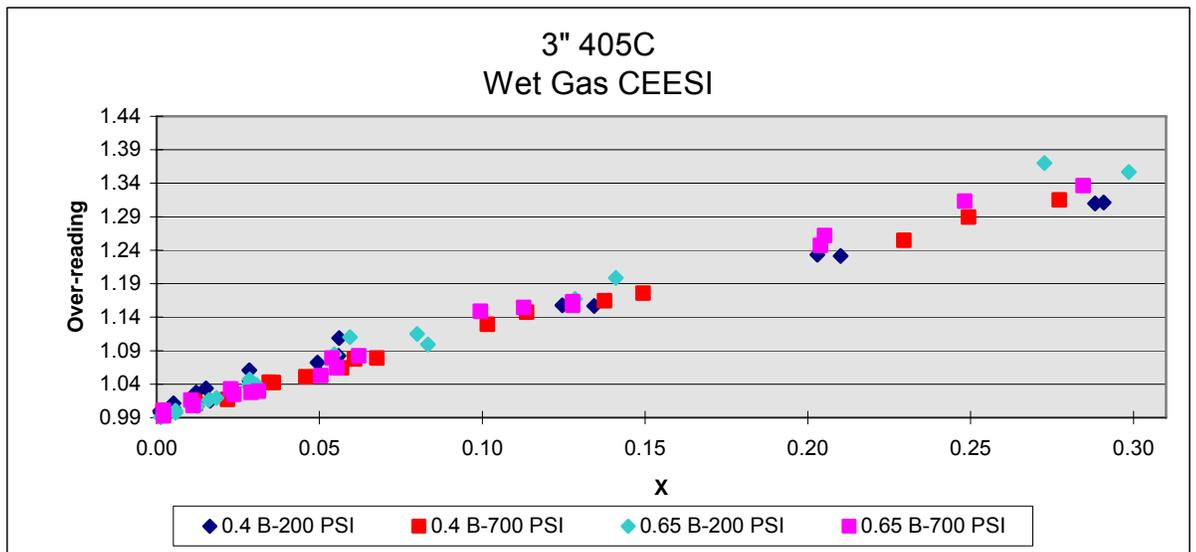
From Figure 8 and 9 it can be observed that both the Rosemount 1595 and the 405C meters follow the same trend with the main source of scatter or variance in the trend being that of the different betas.
