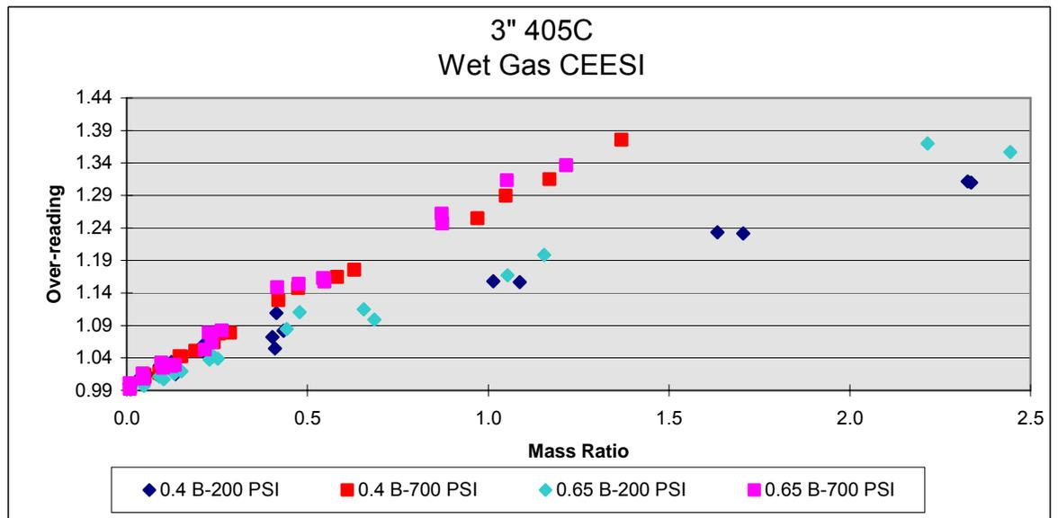
Looking at Figures 8 and 9 there are two distinct trends that follow the pressure of the meters being tested, which is a direct correlation to the density of the gas. In an effort to isolate the meter performance the data is plotted as over-reading vs. Lockhart-Martinelli number.
