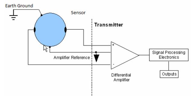
The grounding arrangement is determined primarily by the type of pipe in which the magmeter is installed. The recommended grounding arrangements for conductive unlined pipe, conductive lined pipe, and non-conductive pipe are shown in Figure 2 - Figure 4.
