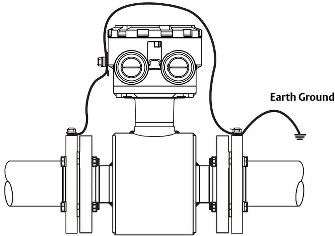
Figure 4. Recommended Grounding for Non-conductive pipe with Ground rings or Lining Protectors
