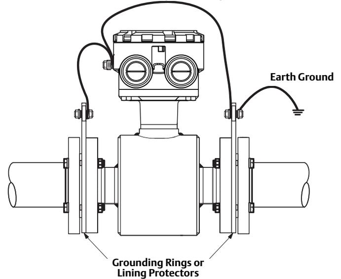
Figure 3. Recommended Grounding for conductive lined pipe with Grounding rings or Lining Protectors<sup>(1)</sup>
