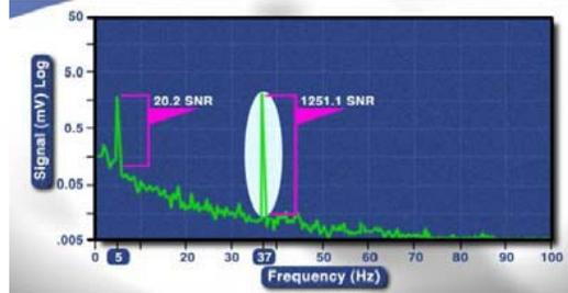
*Increasing coil drive frequency can increase the signal to noise ratio.*
