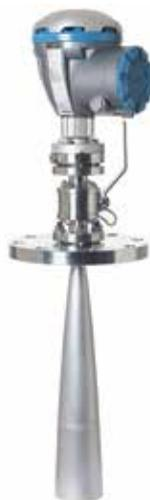
conditions. The pressure seal is equipped with a double-block function, consisting of a quartz/ceramic window and a fire-proof ball valve. A pressure sensor enables volume correction due to vapour for best measurement performance. A reference device function enables measurement verification with the tank in service.
