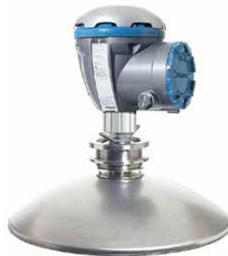
The horn antenna is designed for easy installation on fixed roof tanks, with 200mm (8ins) or larger nozzles. It measures on a variety of oil products and chemicals except asphalt or similar for which the parabolic antenna is recommended.
