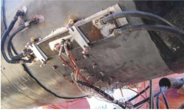
**Figure 1. Sensing pins welded to the external pipe surface as part of an FSM installation in Brazil.**
