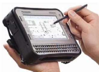
The wireless mobile worker terminal is well suited for industrial environments and is available with a class 1 Div II electrical classification and can include bar code scanners for use with the Operations Management software.
