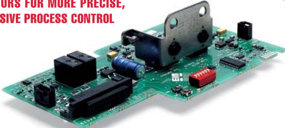
EIM's Digital Futronic control system enables a single electronic module to perform both modulating and positioning valve control from analog control signals. The Digital Futronic module uses digital electronics to improve position control and feedback, and to simplify calibration. Any EIM Series 2000 actuator can be upgraded to Digital Futronic.
