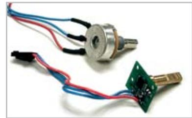
The Futronic system can employ either a standard potentiometer (top), or a contactless Hall-Effect device (bottom) for position feedback.
