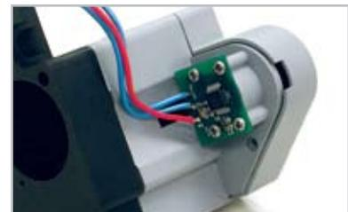
EIM's mechanical dial position indicator (MDPI) equipped with the HPI-M2CP non-contacting feedback device.
