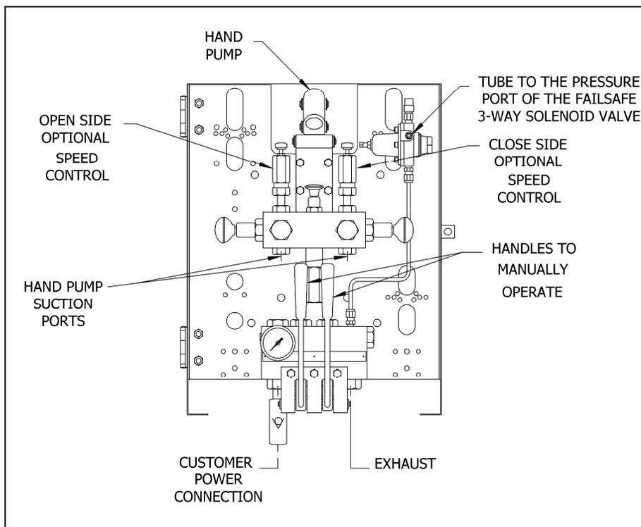
**Figure 9: View of the Control from the Front**
