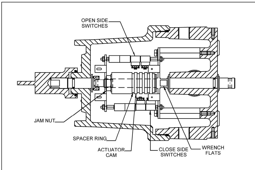
**Figure 15: Cross Section of Limit Switch Assembly**
