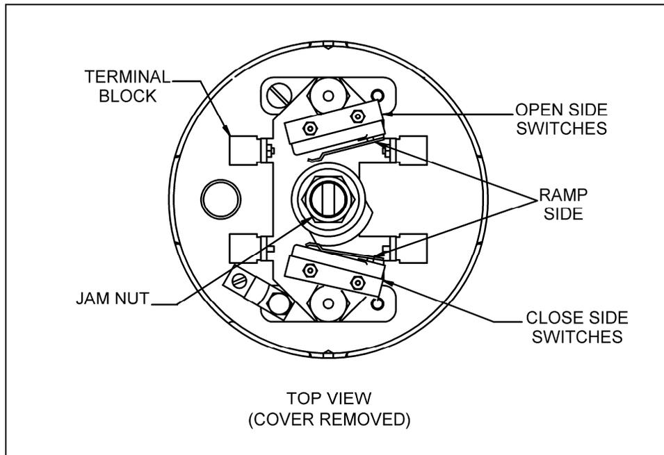
**Figure 16: Top View of Limit Switch Assembly**
